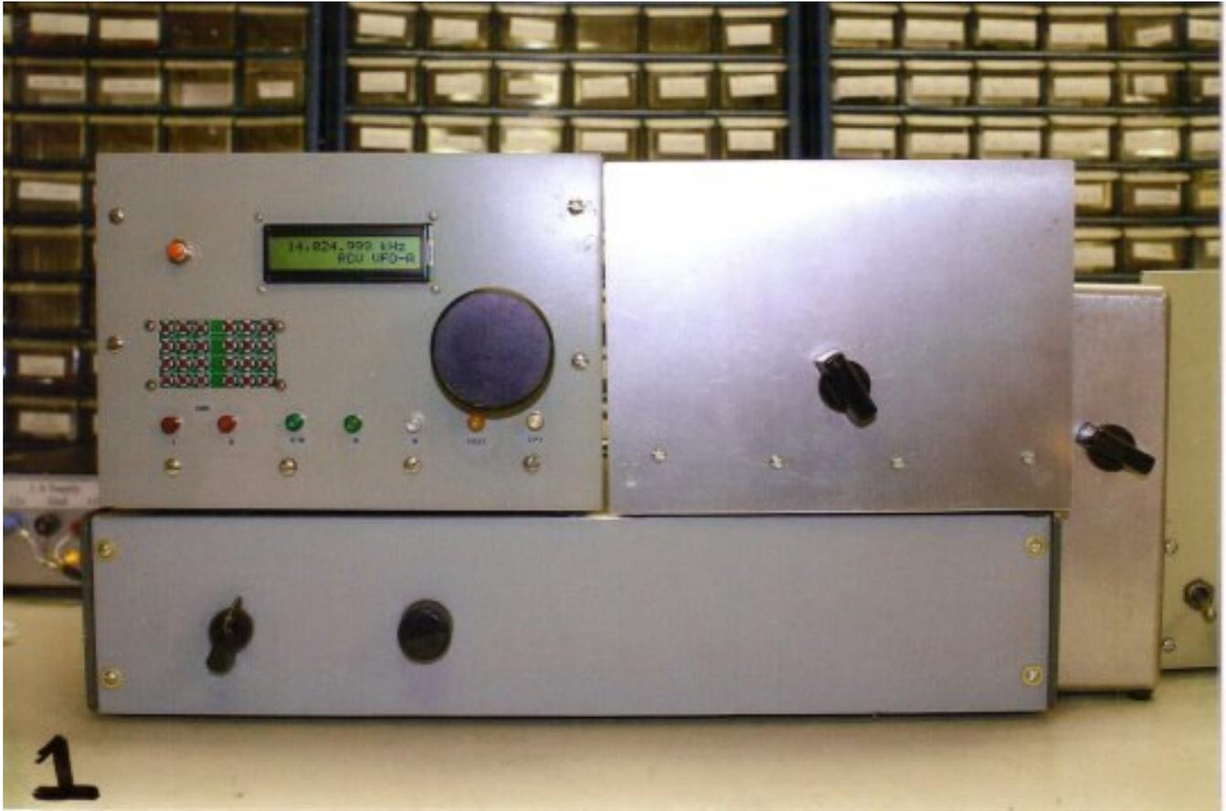
Picture #1: VFO, R2Pro, LP/BC filters, BP filters
