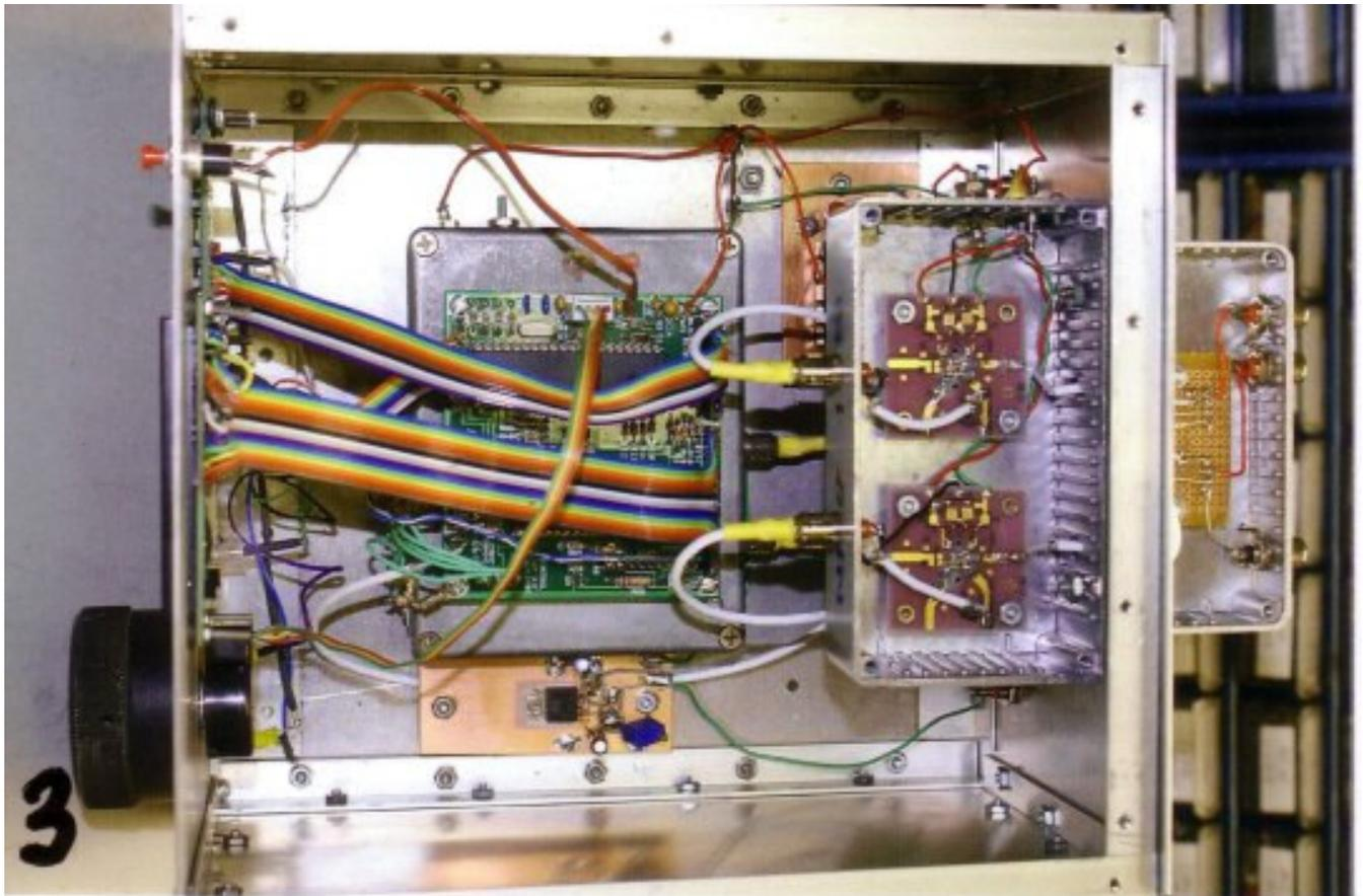
Picture #3: Inside VFO box showing VFO, 6703 amps, TSC-2-1 Splitter/Combiners
